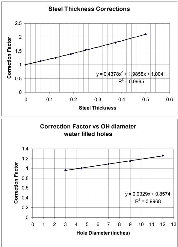
Casing and Water Factors for 2PGA-1000
