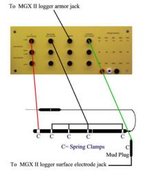
In the absence of the 4RSP-1000 calibrator, a substitute arrangement can be made, by soldering three equal value 5 watt resistors together so that the length of wire between them is as short as possible (less than 1 inch or 2.5 cm). Make connections to this resistor array as indicated in the above diagram. Choose resistor values such that, when multiplied by the proper geometric factor, yield resistivity standards that are with the range of measurement that the probe is currently using.
